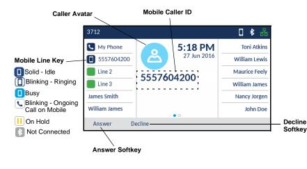
Lift the handset or press the rest = 1000 key, blinking rest = 1000 Bluetooth Line key, or Answer softkey for handsfree operation.
